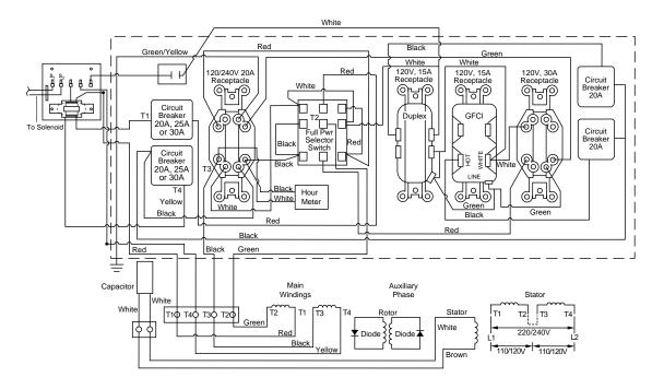
Figure 33 - Wiring Diagram, Model RGH5500AIE
